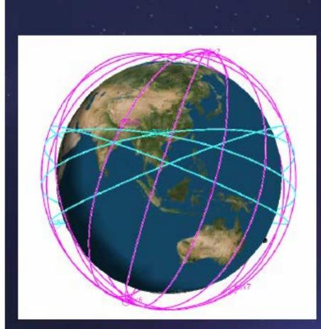
12 Satellites - 2 inclinations Data are distributed more homogeneously COSMIC Occultations-3 Hrs Coverage
