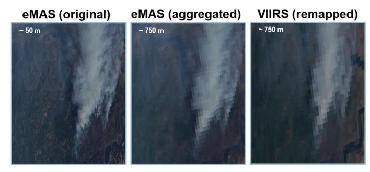
Comparison between RGB images from eMAS and VIIRS sensors. The original resolution of eMAS is 50m and the original resolution of VIIRS is 750m.
