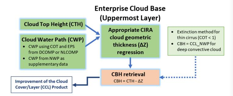
accuracy of] cloud top height." Also, because nighttime satellite cloud data without visible information is relatively unreliable, nighttime collection requires additional data from numerical weather models. Numerical weather models are computer simulations of weather that have drawbacks (accuracy and data gaps) but provide adequate
