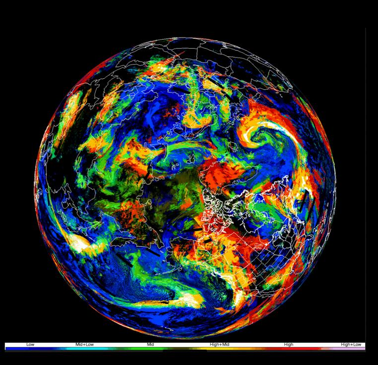
Flight Level-based Cloud Layers RGB. This screenshot of the CIRA Polar SLIDER tool shows flight level-based cloud layers from the improved NOAA Enterprise Cloud Cover Layer Product, including newly expanded Mid+Low, High+Mid, High+Low, and High+Mid+Low (H+M+L) layers.
