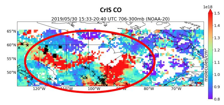
In addition to use in data assimilation for NWP, IR sounders provide data about major air pollution sources, like wildfires, that is complementary to data from other satellite instruments. This figure shows carbon monoxide concentrations across Canada from the CrIS instrument onboard NOAA-20 on May 30, 2019.
