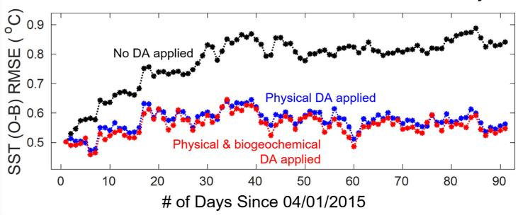
"You can see that adding ocean biogeochemical data assimilation to the physical data assimilation model [red line] has a very small impact on sea surface temperature bias reduction," says Liu. "This was expected," she continues, "because the impact of ocean biogeochemical feedback is created through the lens
