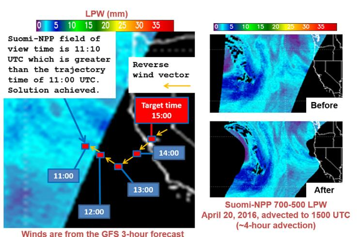
Schematic showing how the back-trajectory method works for advection.
