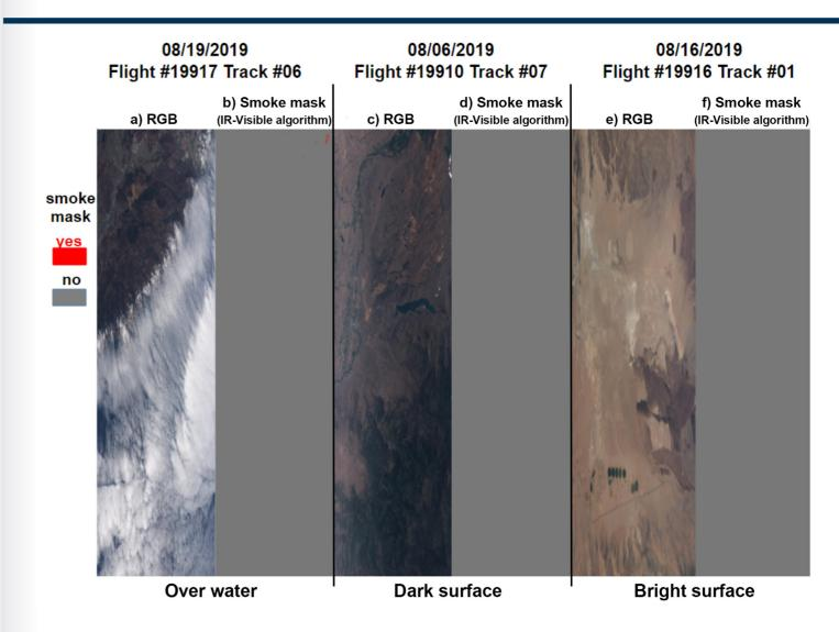
Performance of the Aerosol Detection Product (IR-Visible algorithm path) when applied to eMAS observation tracks that contained no smoke plumes.
