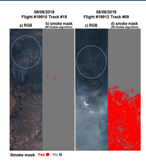
Performance of the Aerosol Detection Product (IR-Visible algorithm path) when applied to eMAS observation tracks that contained thick and thin smoke plumes.
