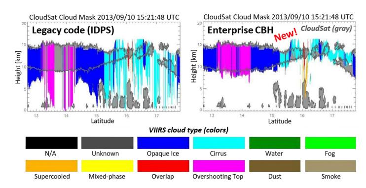
Comparison between the new NOAA Enterprise Cloud Base Height Product (right) and the previous cloud base height product (left) showing improvements with the new CBH algorithm.
