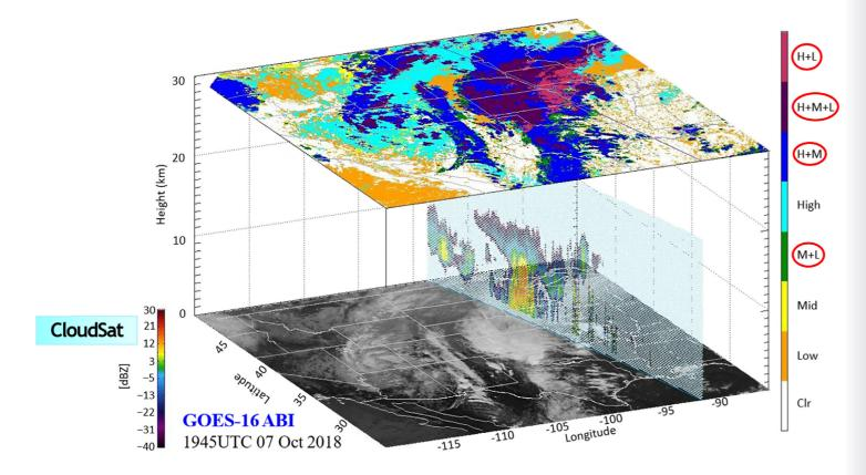
CloudSat overpass showing the addition of cloud top, cloud base, and vertically extended layer information as part of the improved NOAA Enterprise Cloud Cover Layer Product. Newly enhanced layers are circled in red.
