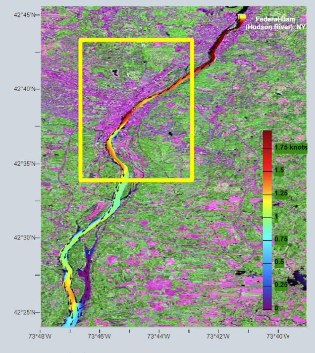
ROLLOVER IMAGE ON LEFT: Comparison of VIIRS ice concentration product data (blue) and Sentinel-2 imagery (gray) from the River Ice Mapping System that illustrates ice motion for a downstream portion of the Hudson River in New York on February 26, 2022. Right: Velocity values in the Hudson River on February 26, 2022, from the Stevens Flood Advisory System (https://hudson.dl.stevens-tech.edu/sfas/).
