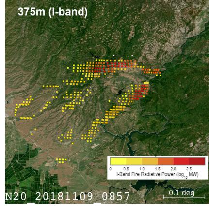
NOAA-20 VIIRS Fire Radiative Power (FRP) measured by the VIIRS M-band (top) and I-band (right) for the Camp Fire in California on November 9, 2018.
