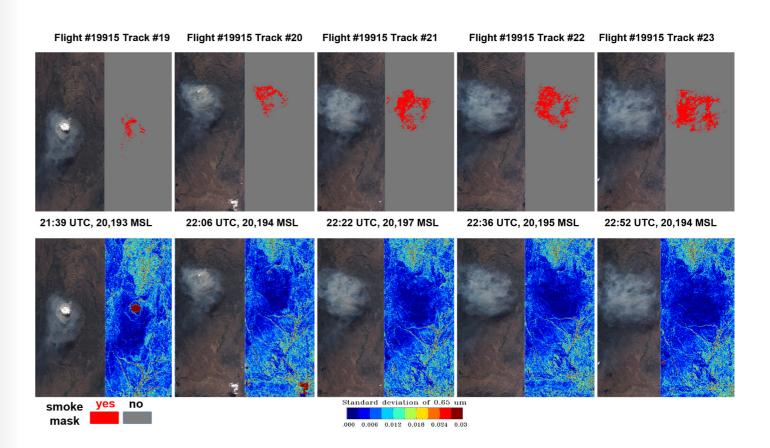
Top row: Performance of the Aerosol Detection Product (IR-Visible algorithm path) when applied to eMAS observations of the Sheridan Fire that were taken minutes apart on August 15, 2019. Bottom row: Standard deviation showing that smoke plumes are mostly uniform.
