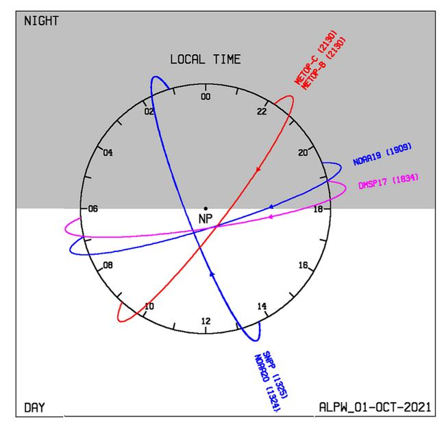
This "clock diagram" shows the local time of polar orbiting satellites used to produce the ALPW product. Note the different orbits that contribute to irregular observation times.
