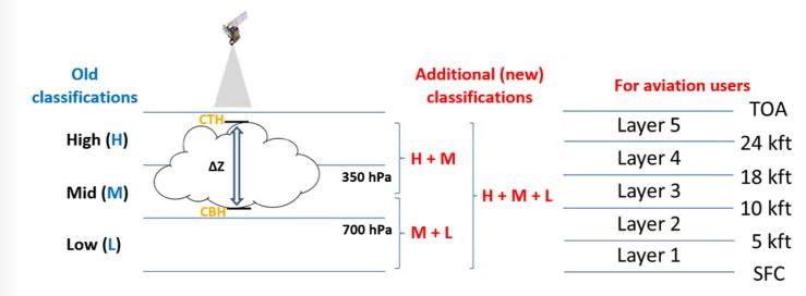
Expansion of cloud classifications from three to five flight-based level layers.
