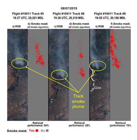
Performance of the Aerosol Detection Product (IR-Visible algorithm path) when applied to eMAS observations of the Williams Flats Fire that were taken minutes apart on August 7, 2019.
