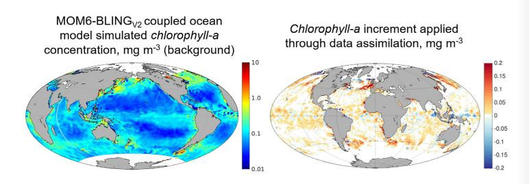
Left: Simulated chlorophyll-a concentration from the coupled MOM-BLINGV2 component of the coupled global UFS application (snapshot of background at 12 hours on May 1, 2019). Right: Chlorophyll-a increment applied through JEDI-based data assimilation using a 3DVar scheme covering 2019-2022 and is a 24-hour data assimilation cycle. Both the coupled global UFS application and the data assimilation application have a resolution of 0.25 degrees for the global ocean.
