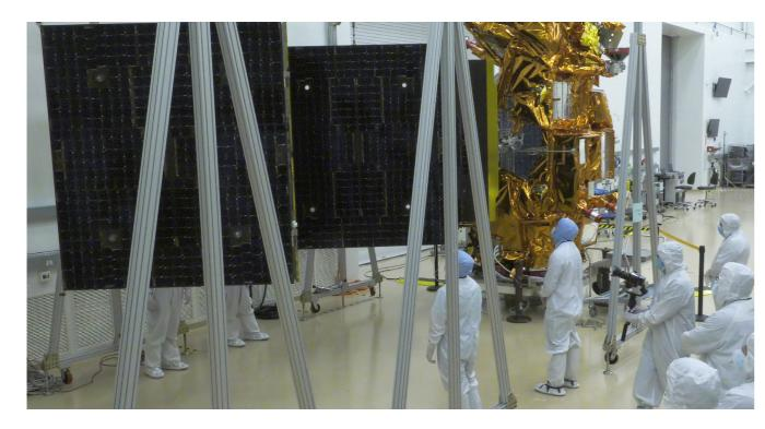
On July 26, in a clean room at the Northrop Grumman facility in Gilbert, Arizona, NOAA's JPSS-2 satellite let out several loud pops as each of the five panels of its solar array detached from the body of the satellite and then unfolded, stretching out to its full 30-foot length. Under each panel, an engineer clad in a bunny suit flashed a thumbs up as latches clicked into place.
