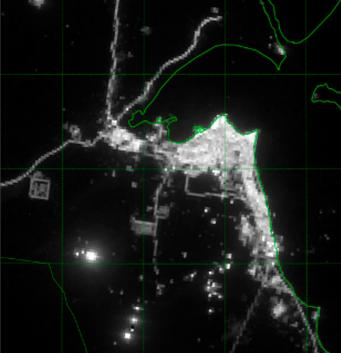
Nighttime city lights over Kuwait City captured by the DMSP OLS sensor at 3-5 km resolution (left) and the VIIRS Day/ Night Band at 742 meter resolution (right).
