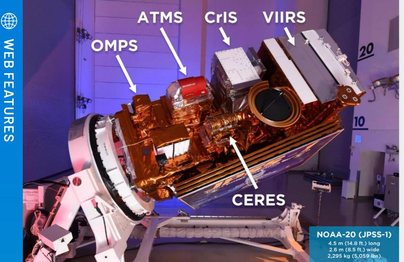
ATMS and VIIRS are part of a suite of instruments on the NOAA-20 satellite. Credit: Ball Aerospace.
