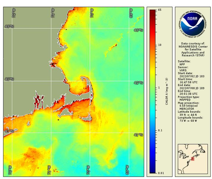
Example output from the VIIRS (Suomi-NPP) 7-day chlorophyll-a product for July 2, 2022 to July 8, 2022 for the Massachusetts and Rhode Island Bays. The product is processed with the NOAA OC3 algorithm and near-infrared (NIR) atmospheric correction. Source: NOAA CoastWatch East Coast Node.
