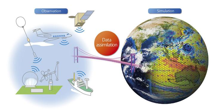
Data assimilation is the bridge between real-world observations and computer simulations. Observations from many sources increase the accuracy of weather forecasting through numerical weather prediction models. Source: RIKEN AICS.
