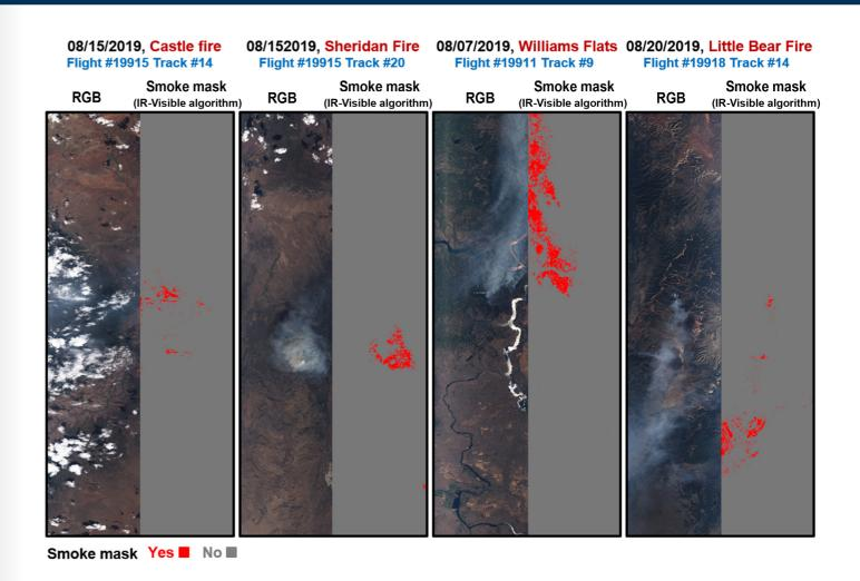
Performance of the Aerosol Detection Product (IR-Visible algorithm path) when applied to eMAS observations of wildfire events during the FIREX-AQ field campaign.
