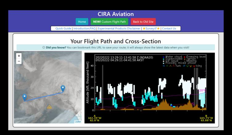
Screenshot of CIRA's Cloud Vertical Cross-section product website that allows users to select routes of their choice on a map to create a custom cross-section displaying cloud phase, altitude, terrain, turbulence, and icing information.
