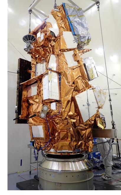
The JPSS-2 satellite in the vibration chamber at the Northrop Grumman facility in Gilbert, Arizona. Credit: Northrop Grumman
